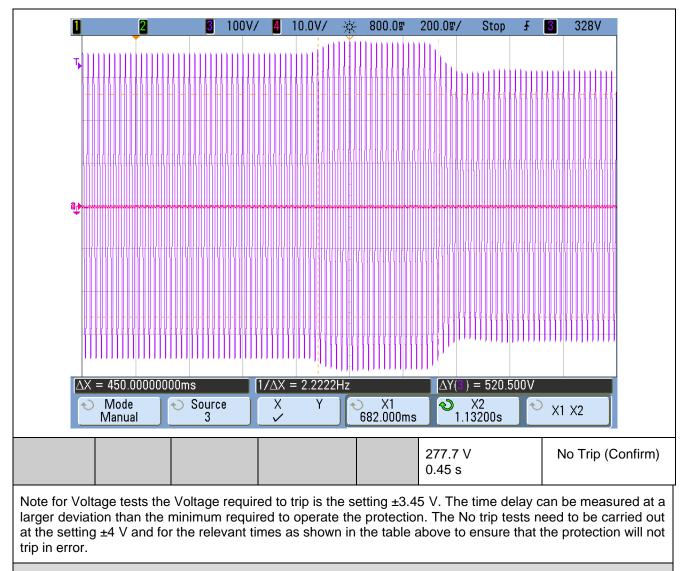
**8.Protection – Loss of Mains test:** These tests should be carried out in accordance with BS EN 62116. Annex A.7.1.2.4.
